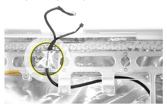
3. Near the middle of the rear housing, remove the two T8 screws on the cable guide
